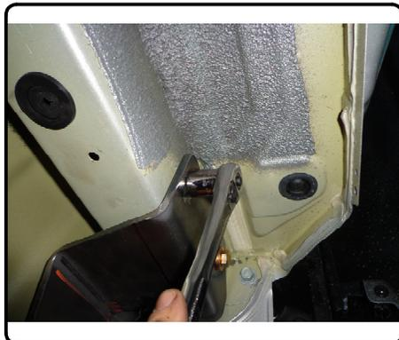
5. First torque the 3/8" U-bolt to 30 lb-ft and then the M10 bolts to 51 lb-ft.
