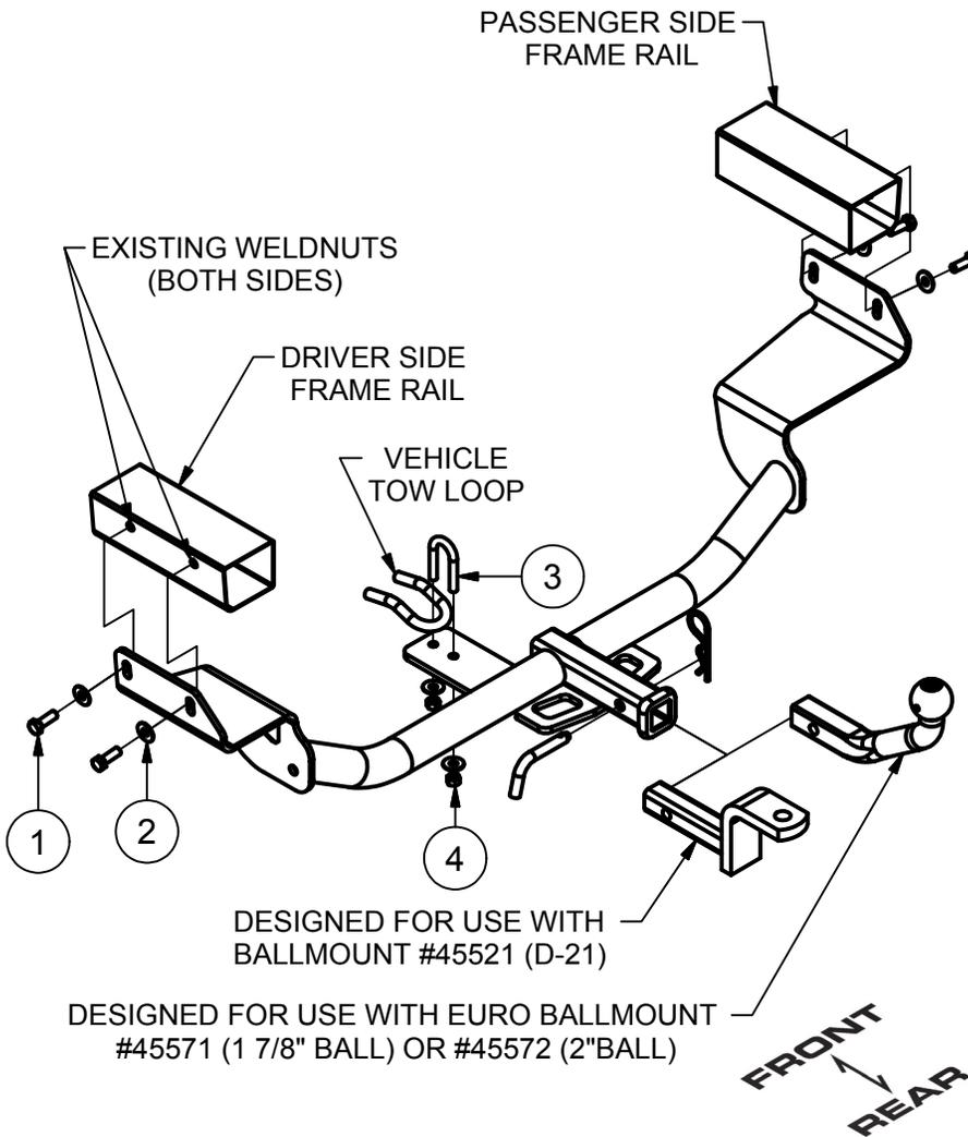
1. Remove underbody panel on the driver side of vehicle by removing (4) M10 nuts and (3) push fasteners. Return fasteners and underbody panel to customer.
