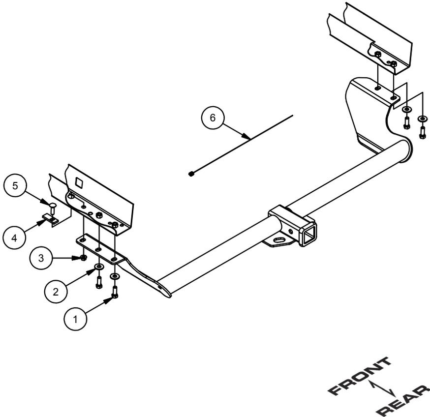
1. If present, remove (5) fasteners and the plastic fascia covering the driver side frame rail. Return fasteners and plastic fascia to owner. **Note:** You may trim fascia and reattach after hitch installation.
