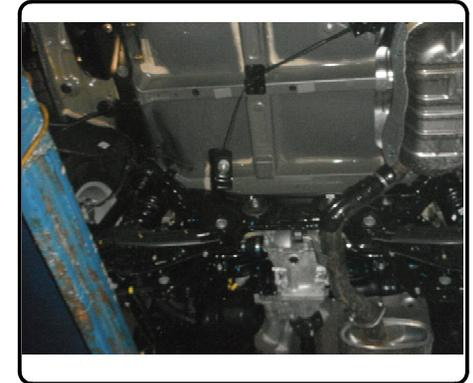
2. Temporarily remove underbody panel on driver side of vehicle by removing (5) screws and (2) nuts. Retain screws for reinstallation of panel.
