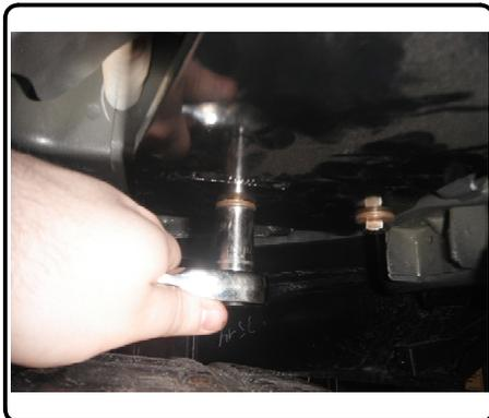
8. Raise exhaust back into position and reattach rubber isolators removed in Step 2.
